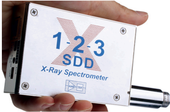
Figure 2.5.1: Ametek X-123SDD Complete X-Ray Spectrometer with Silicon Drift Detector (SDD)
